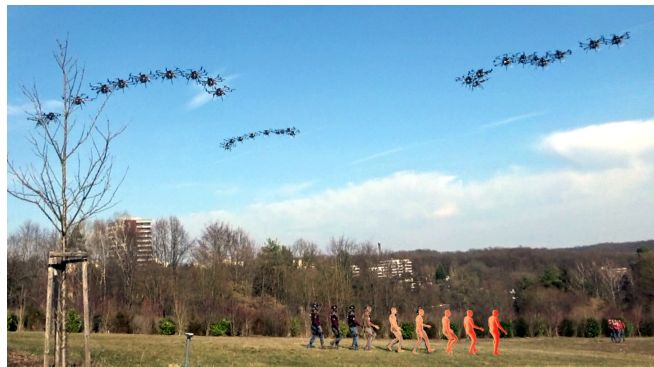
Fig. 1: 3D markerless motion capture from fully autonomous micro aerial vehicles (MAVs) with on-board cameras. Multi-exposure image shows the trajectory of the MAVs and the 3D body pose and shape projected onto an image frame from an external camera.
