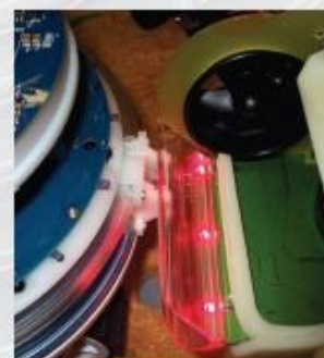
Above: current Hand-bot prototype. Above right: attachment ring and mechanism on Foot-bot. Right: close view of the attachment between Foot- (left) and Hand-bot (right).
