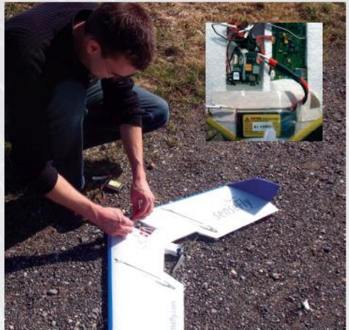
Clockwise from above left: current model of flying robot SMAV. Severin Leven replacing the battery on one of the SMAV robots. Inset: SMAV control box Linux board on right, autopilot on left and battery in front for easy replacement. Current prototype of the Eye-bot.
