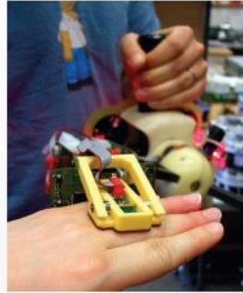
Far Left: Hand and Foot-bot with roboticist Micheal Bonani. Center: Hand-bot grips with 4kg pressure any object which activates the sensors. Above: close view of the Hand-bot gripper.
